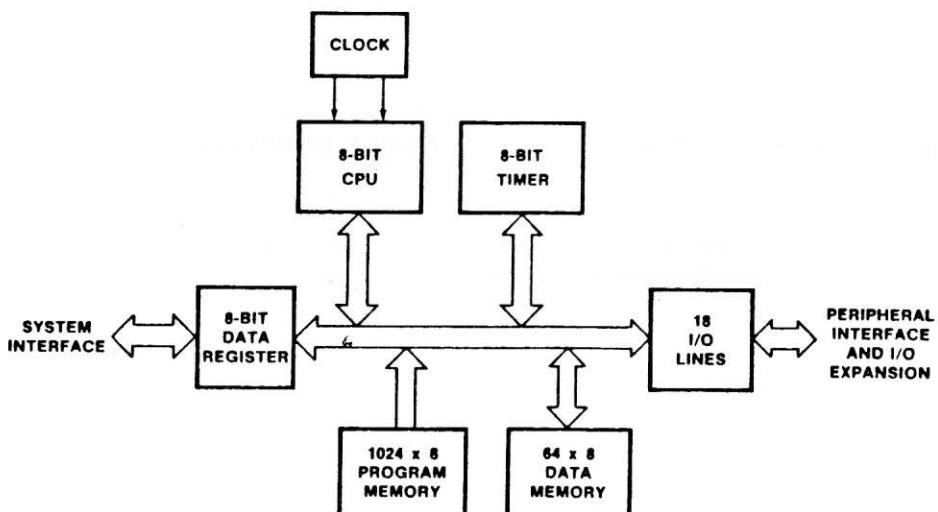
Figure 2-1. UPI-41 SINGLE CHIP MICROCOMPUTER
