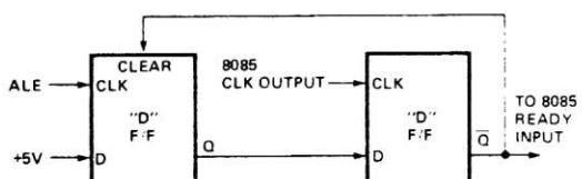
**FIGURE 7. GENERATION OF A WAIT STATE FOR 8085 CPU**
