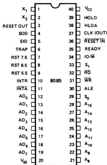
Figure 1. 8085 PINOUT DIAGRAM
