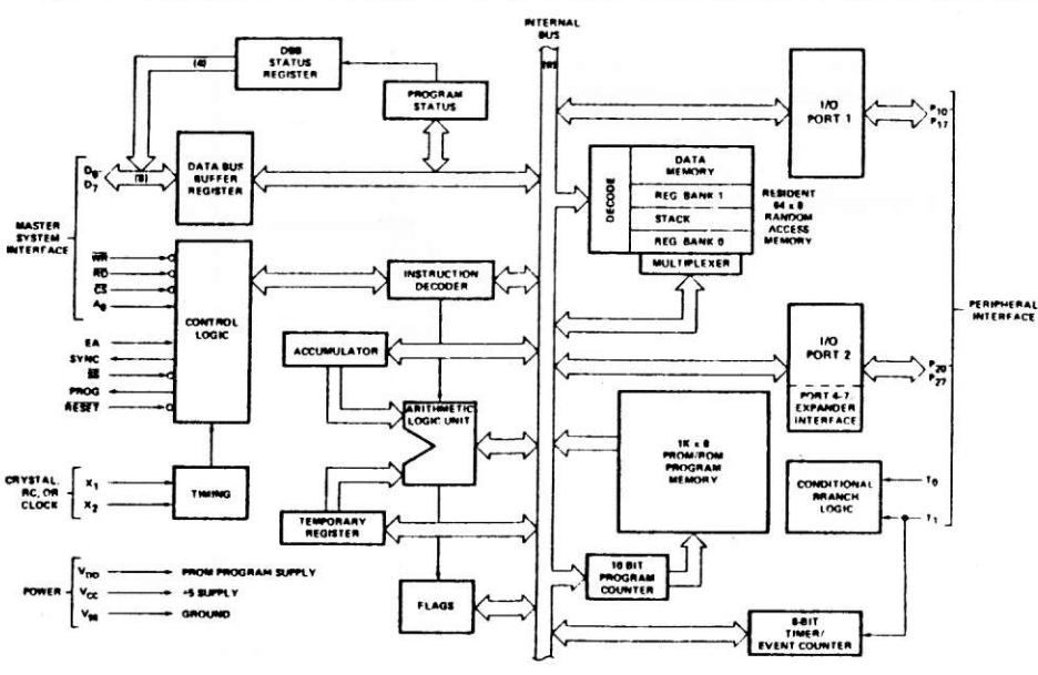
Figure 2-4. UPI BLOCK DIAGRAM
