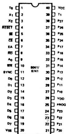
Figure 2-2. PIN CONFIGURATION
