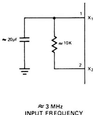
RC Mode causes a large drift in clock frequency because of the variation in on-chip timing generation parameters. Use of RC Mode should be limited to an application, which can tolerate a wide frequency variation.
