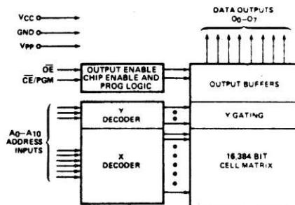
\*Pin 18 and pin 20 have been renamed to conform with the entire family of 16K, 32K, and 64K EPROMs and ROMs. The die, fabrication process, and specifications remain the same and are totally unaffected by this change.
