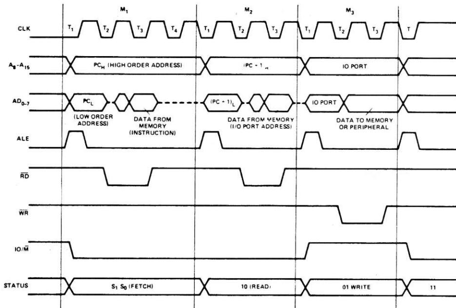
FIGURE 2. 8085 BASIC SYSTEM TIMING.
