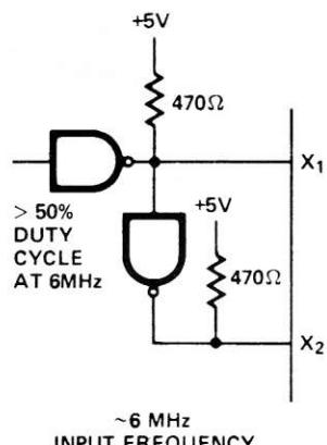
This circuit may be used when the clock input has > 50% duty cycle at 6MHz.
